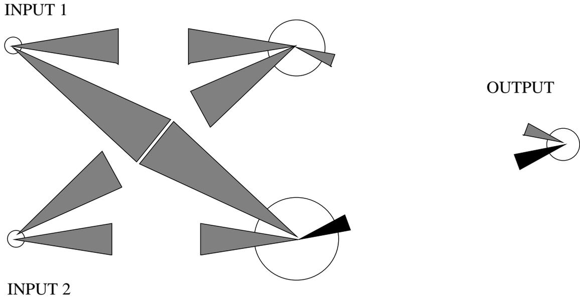
Figure 6: **A bond diagram.** The diagram depicts the network shown in Figure 1. The size of a unit indicates the magnitude of its bias. Positive and negative weights are shown as light and dark shaded bonds, respectively. The magnitude of a weight is indicated by the amount of the bond which is shaded.
