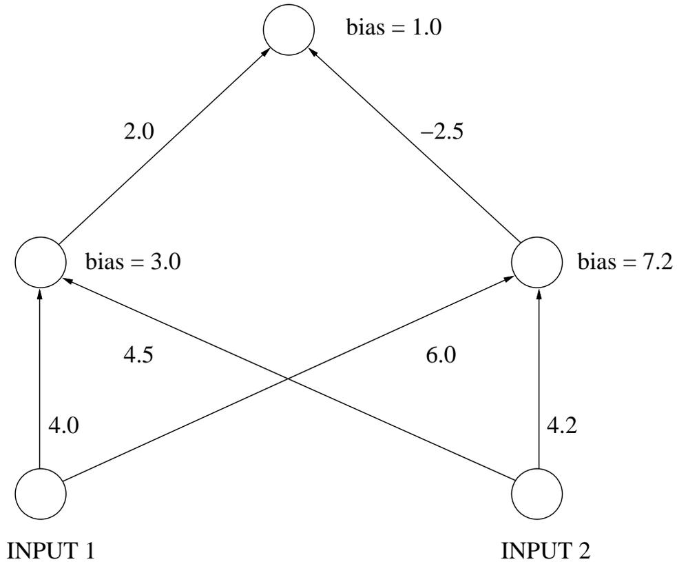
Figure 1: **A simple artificial neural network.** When given input values which are either 0 or 1, this network implements the XOR function. The network can be thought of as returning *true* when the activation on the output unit is greater than 0.5.
