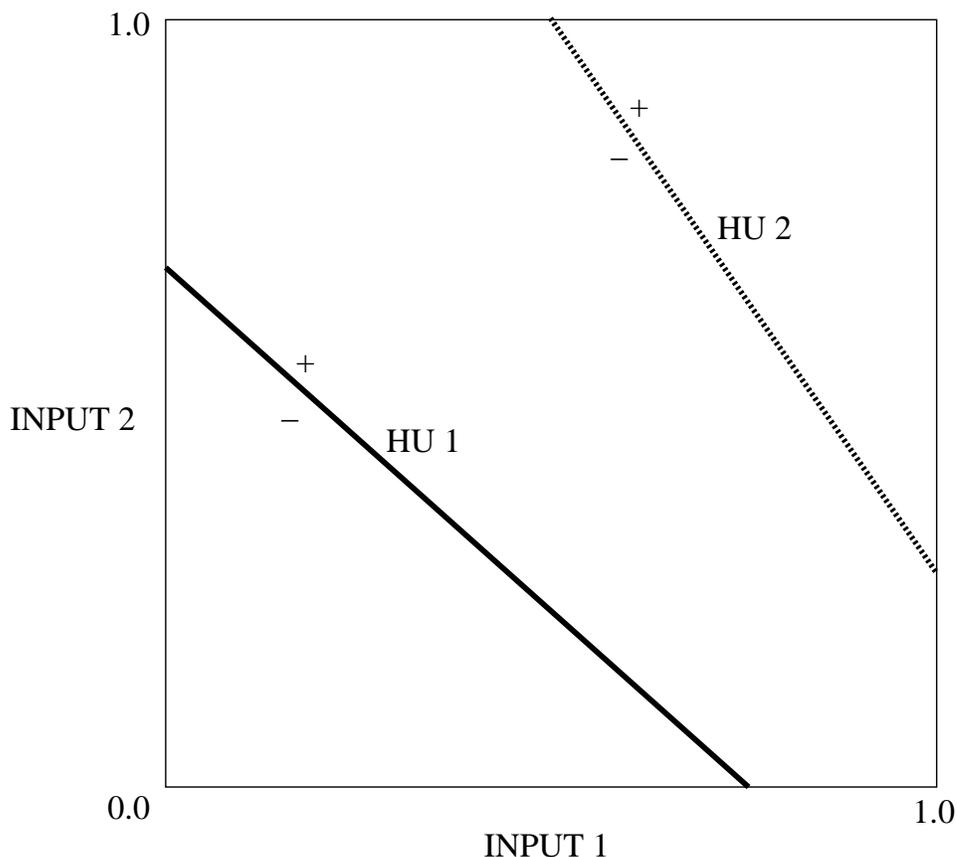
Figure 7: **A hyperplane diagram.** The diagram shows the hyperplanes defined by the two hidden units in Figure 1. HU1 refers to the leftmost hidden unit in Figure 1, HU2 refers to the rightmost hidden unit.
