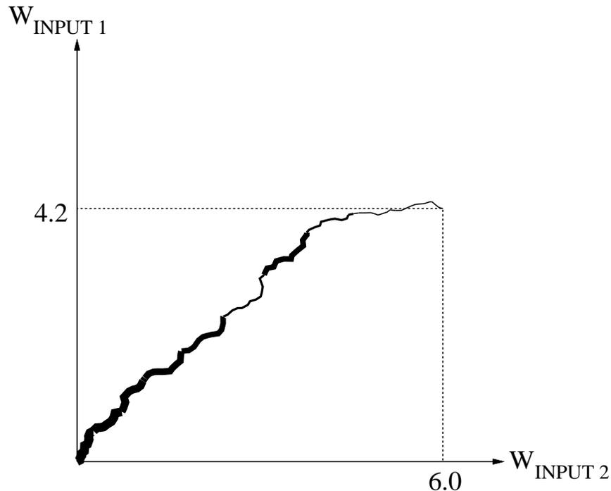
Figure 9: **A trajectory diagram.** The diagram depicts the trajectory, over a hypothetical training session, of the rightmost hidden unit in Figure 1. The trajectory is plotted in the space defined by the two weights impinging on this hidden unit. The thickness of the trajectory line indicates the network error along the trajectory.
