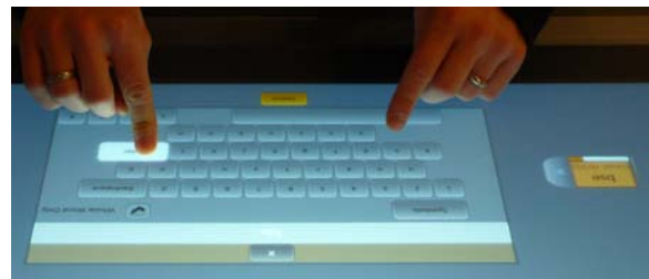
Figure 2: Interaction starts with a search. Each user is assigned a color, which is reflected in the search button (top) and keyboard (bottom).
